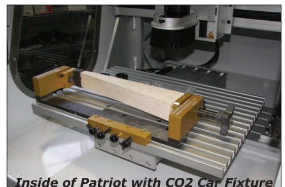
Inside of Patriot with CO2 Car Fixture
