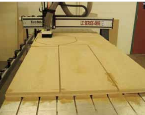
Figure 1. Techno machine cuts an octagonal tabletop and rectangular tops at Vermont Correctional Industries.
